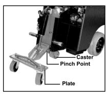
Note: Make sure the plate is parallel with the floor so the caster swivels freely.
