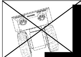
CAUTION: MACHINE IS BACK HEAVY. DO NOT RUN ON STEEP INCLINE--THIS COULD CAUSE MACHINE TO TIP OVER!
