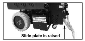
**Figure A** Correct slide plate setting with a steep cutting head angle.
